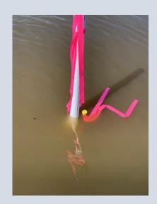
Kelly Carr, PLS "Photos are attached of a property corner set on a recent survey in the middle of a lake in Ballard County. The 5/8 inch rebar set is 10 feet in length and marked with 2 inch PVC. The corner set delineates property that was once part of an Illinois Central Railroad Cairo District Right of Way constructed in the early 20th century. Use of the Rail line was discontinued in 1957. Field crew pictured are Ethan Carr, LSIT and Emily Landis."
