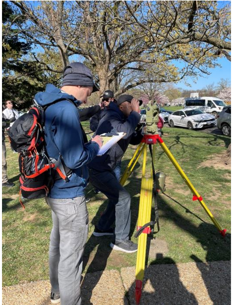
Left to Right: Maximilian Paul and Name Withheld Per Student Request use a Wild T-2 Theodolite to sight the top of the Washington Monument, as part of the Triangulation Challenge, Day 2 of the 2023 Young Surveyor Network, Student Competition
